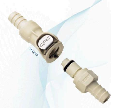
The 1/4" flow polypropylene PLC12 offers many of the same configuration options as the PLC. The polypropylene material adds greater chemical resistance for more demanding applications. PLC12 couplings are also gamma sterilizable. PLC12 coulings are also gamma sterilizable and available with optional RFID (Radio Frequency Identification) capability (see page 96).
